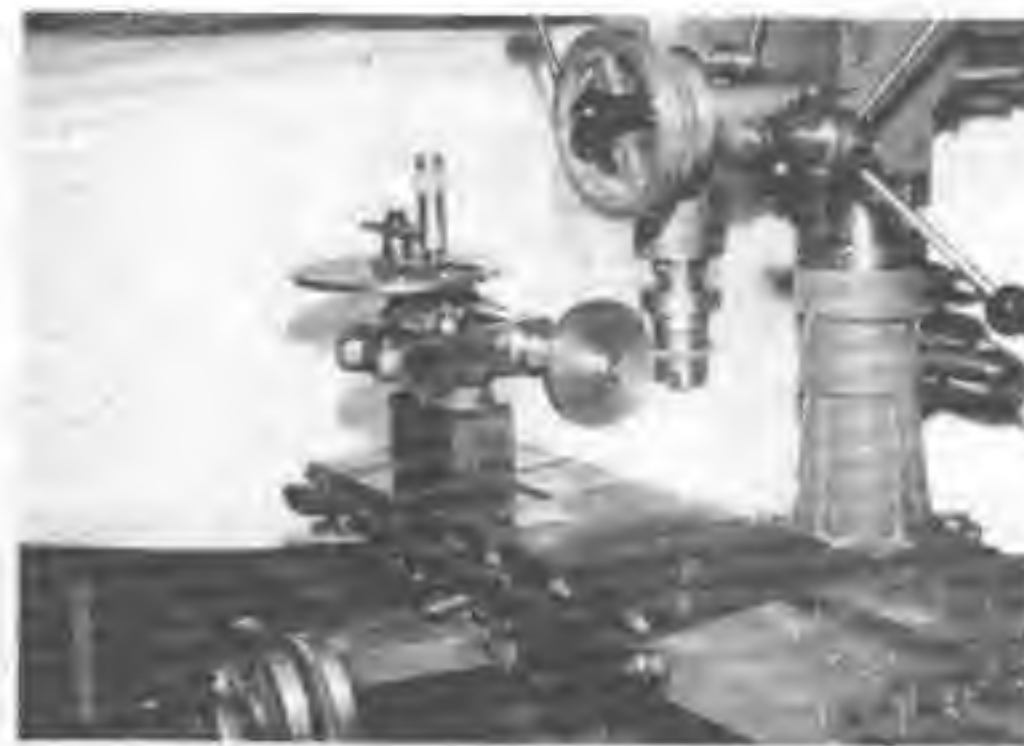
Fig. 64 Cutting a spur gear on the vertical miller. The dividing head is mounted on a raising block.
